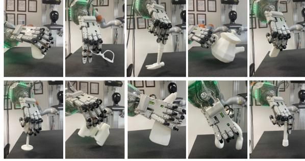
**Fig. 7.** Grasping tasks for 3D printed rigid objects. Top row, left to right: bottle, glasses, hammer, teapot, cell phone. Bottom row, left to right: wine glass, binoculars, cleanser bottle, headphones, flashlight.
